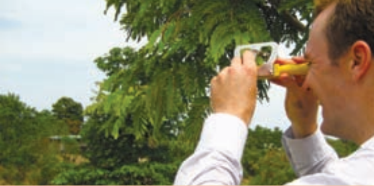
Simon Douse uses an Abney level to survey a potential crossing point
